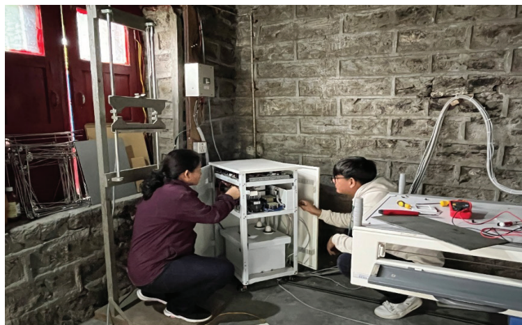
Fig 1: We successfully restored the X-ray CR system at Manang Hospital, which had been non-functional for a year. We addressed issues with exposure, expired software licenses, and a damaged PC.
